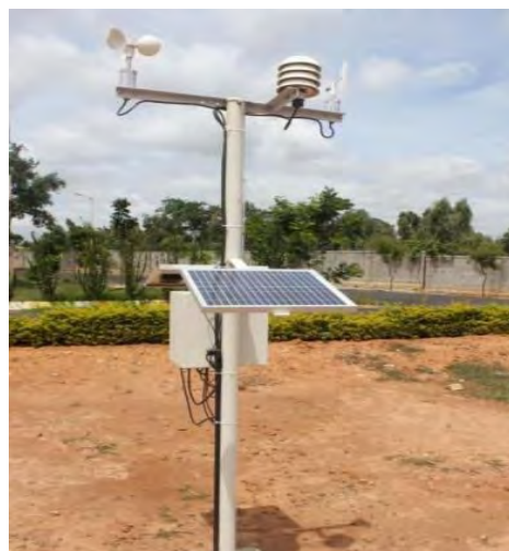
Telemetric Weather Station
