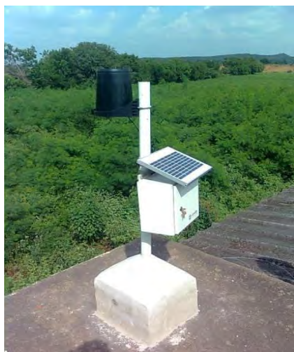
Telemetric Weather Station Telemetric Rain Gauge
